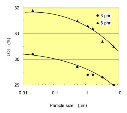
As the effectiveness of a flame retardant varies of according to the size of antimony trioxide, as explained above. Therefore, if a highly effective flame retardant is required, special attention should be paid to the size of antimony trioxide particles.
